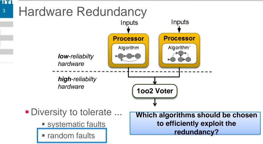
Inherent fault masking at algorithm-layer
